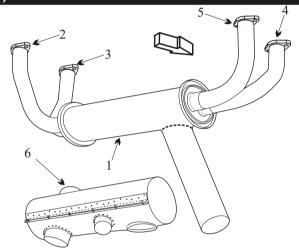
AD 74-06-02 Applies to STC Avcon Industries muffler. Replace muffler.
