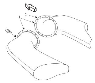
Inspect exhaust where flanges attaches. The exhaust nozzle usually cracks from the inside in this area.
