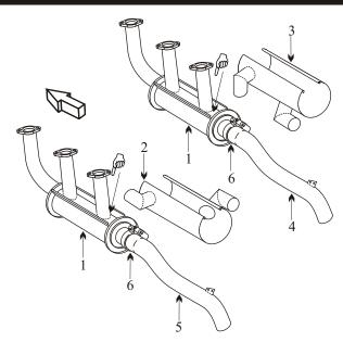
Inspect the area where riser attaches to the body of the muffler for cracks.
